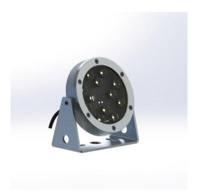
Waterproof floodlight that integrates 12 Power LEDs in an anodized aluminum or 316L stainless steel body. With its specific optics, it provides an extensive or intensive monochromatic luminous flux according to the applications
